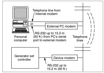
Figure 11 Remote Single Connection
