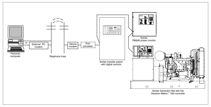
Figure 13 Power System Communication Network Configuration Using Telephone Lines
